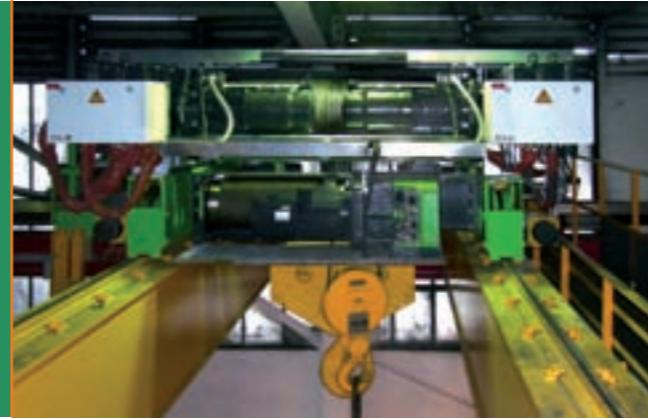
The 35t winch type SHWF with a wire rope hoist type SH as auxiliary hoist in the foreground.
